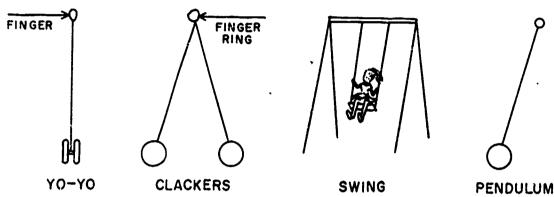
All these systems will run down unless supplied with energy. How is the energy fed in? A good starting system is the clock pendulum on a rigid rod.
