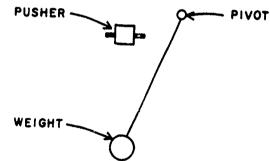
A linear actuator or one of the rotating joints can be used as a "pusher". A simple experiment will show the need for a good phase relationship. When this is understood, proceed to the flexible string and finally the interesting case of the swing in which the source of energy is carried by the pendulum.
