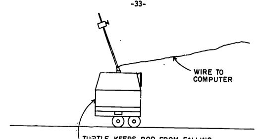
TURTLE KEEPS ROD FROM FALLING BY MOVING FORWARD AND BACK. POTENTIOMETER IN HINGE PROVIDES INFORMATION FOR FEEDBACK.
