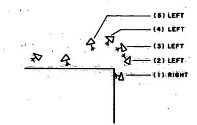
To circumnavigate the room from the inside one could use FRONTTOUCH to know when to turn. A small extension of the procedure could enable the turtle to find a door and escape from the room. Or explore a maze. Or ...
